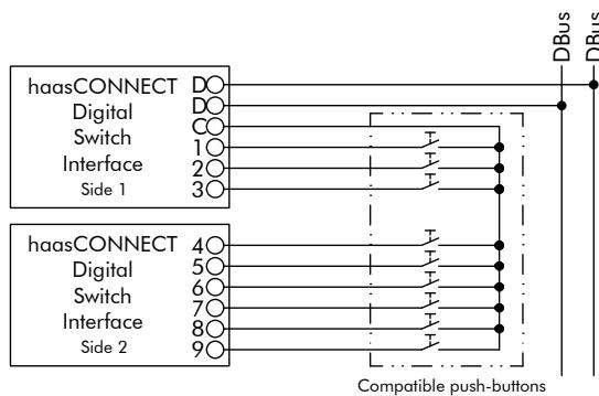
DBus - connections to haasCONNECT Digital Controller Digital bus channel
